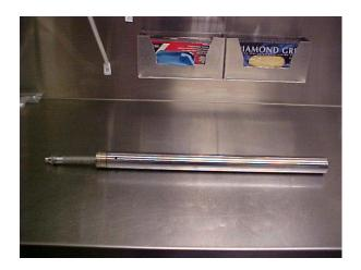
2. The fork tube must have outer lip ground off as seen below, until there is a flat even surface all the way around. Grind off only about 1.5mm to 2mm off the end of the fork tube. **Preferred method is to use a lathe to accomplish this**.
