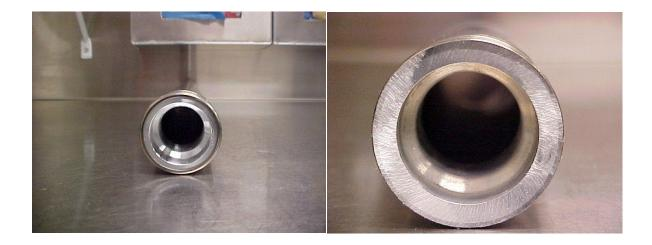
3. Knock out the parts inside the bottom of the tube by dropping a 24 mm socket down into the tube. Deburr and thoroughly clean the tube. Reassemble tube with leg as it was disassembled. Replace oil seal, and bushings as needed.
