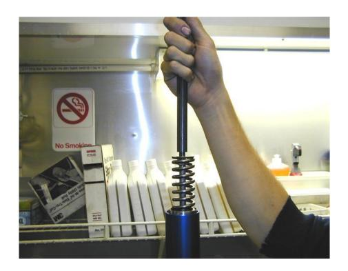
Once the tool is securely attached to the damper rod stroke the damper rod up and down until smooth. When there is air the cartridge the stroke will be notchy feeling. Once the cartridge is bled the stroke will be smooth.
