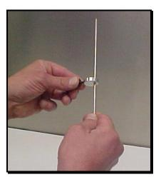
2. Hold the adjustable height ring on top of the fork tube so the oil level rod is inside the fork. Fork needs to be fully collapsed, with the springs and spacers out to set oil level.
