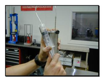
3. Pull the plunger on the syringe until no oil is being removed. Oil level is set.
